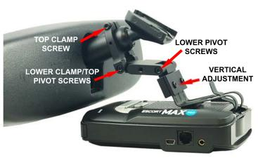
7 - Install the RD onto the mount. Make the necessary adjustments as shown above. Using the vertical adjustment, we recommend you adjust the RD as close to the bottom of the mirror as possible. The spring clip holding the RD is designed to flex downward to allow access to the RD buttons as shown below in step 10.
