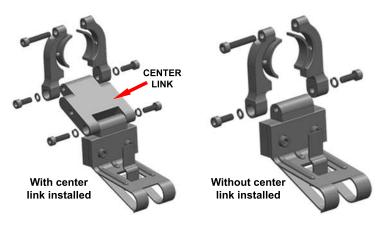
**6** - The center-link may be removed if an overall shorter mount length is needed, depending on your rear view miror and desired position for the RD.
