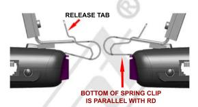
2 - The bottom of the spring clip must be parallel with the top of the RD to slide in and out. Slide the RD onto the spring clip as far as it will go. Let go of the release tab to secure the RD onto the mount. Before installing the mount onto your rear view mirror, remove and install the RD a few times so you can observe how the spring clip functions.
