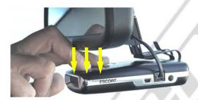
10 - To access the buttons of the RD you will need to gently push downward on the front of the RD with one finger and push the desired button with another finger. Then allow the RD to return to it's original position by gently letting it spring upward. When accessing the buttons, be sure to push the RD downward just enough for your finger to fit between the RD and mirror.
